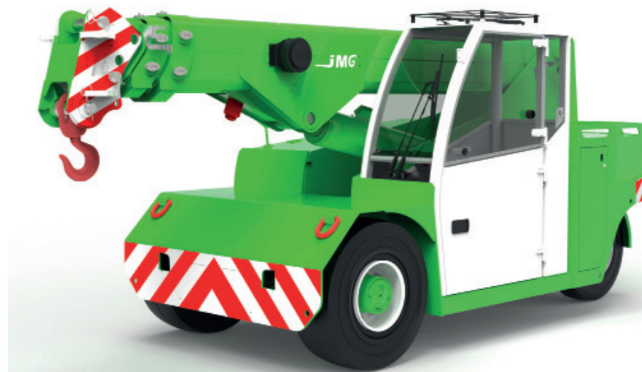
MC 85 (metric) Max Capacity 8,500 kg
