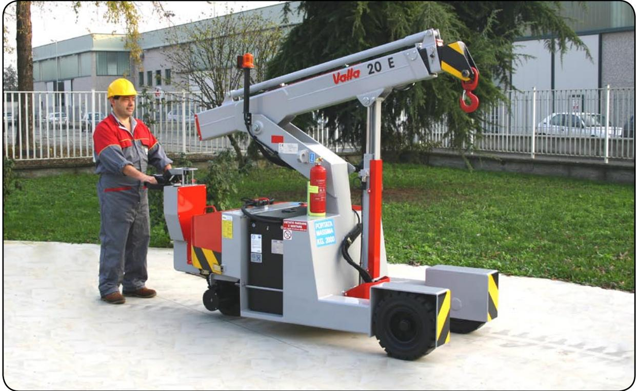
**PROPULSION:** 2 kW - 24 V AC fanned reversible electric motor fitted with electronic speed control. Disk brake on drive wheel electrically operated. Equipped with dead man cut out. Reduction between motor and wheel by gears in oil bath. Max speed 3,5 Km/h.
